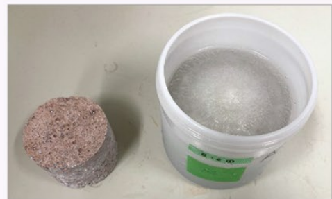
Immerse the test sample in water, freeze it, and take CT scans with the container.
